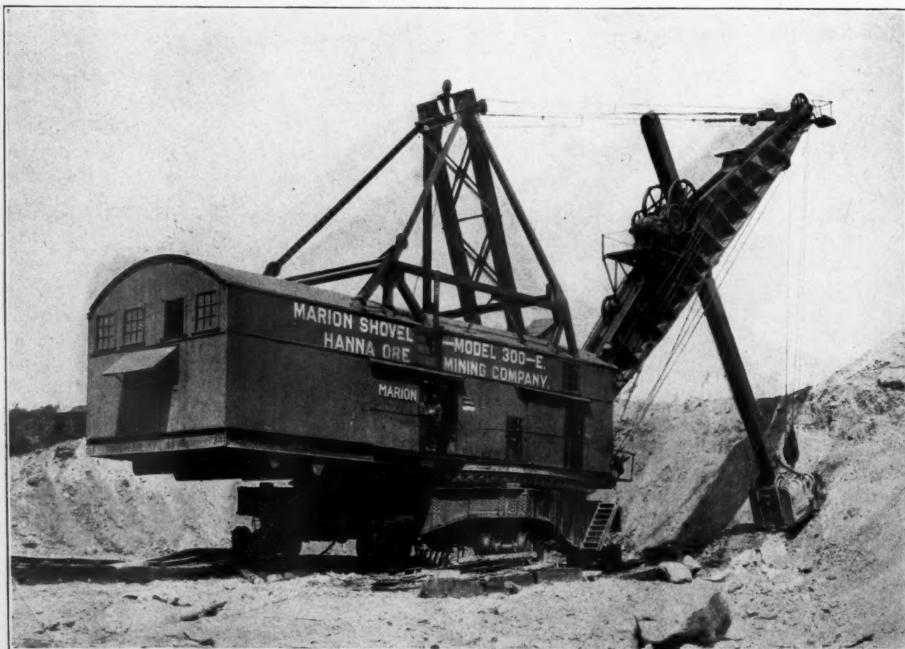
Large Revolving Railroad-Type Shovel With Four Trucks and Special Double-Flanged Wheels
